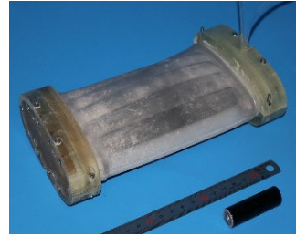
Fig. 11 Overview of the Prototype Model of the Jamming Pillow Mechanism
